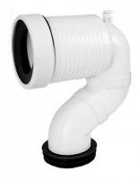
Pan connectors come in different sizes and offsets to suit any toilet model enabling the trap outlet to reach the pipe, as in most cases, especially in replacement situations the soil or drainage pipe cannot be moved to accommodate the new toilets connection set-out measurements.
