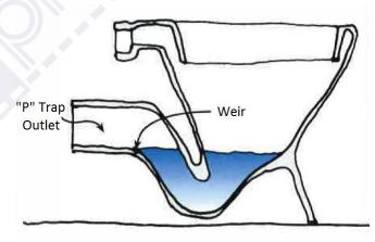
Pans are designed to connect to a soil pipe (drain pipe) through the
